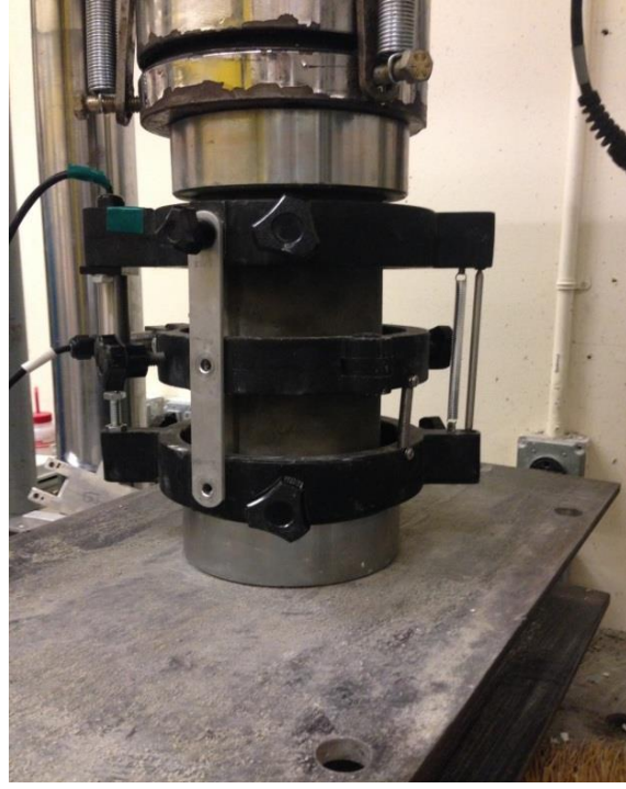
Figure A-2: Cylinder Testing - Modulus of Elasticity
