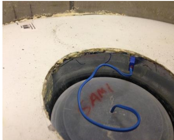
Figure 7: Middle Thermocouple Placed and Plugged In
